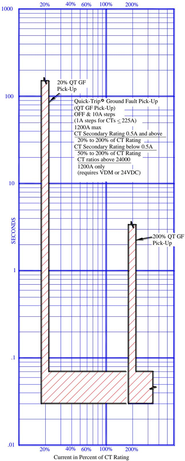
Quick-Trip<sup>®</sup> Ground Fault Time Current Curve
